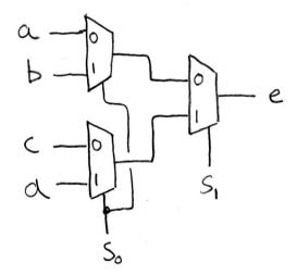
The first layer of muxes uses the  $s_0$  input to narrow the four inputs down to two, then the second layer uses  $s_1$  to choose the final output.
