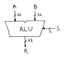
when S=00, R=A+B when S=01, R=A-B when S=10, R=A and B when S=11, R=A or B = 11, R=A or B
